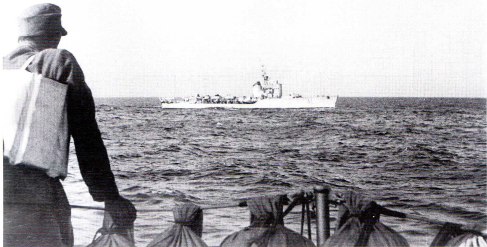
Above: A life-jacketed Gebirgsjäger looks over the rail at the escorting Italian destroyer en route for Crete. The destroyer is the Lupo which was a Quarnaro boat of the 'Partenope' class, with a displacement of some 679 tons and a crew of 94. Alexander Turnbull Library — DA1308
